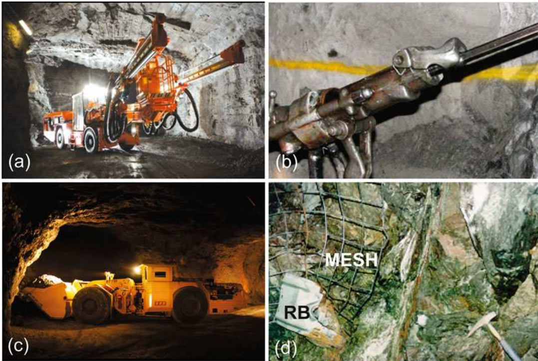
Fig. 2.3 Examples of the underground machineries and equipment: (a) two beams Jumbo; (b) air leg; (c) LHD truck; (d) underground working supported by meshing and rock bolting (RB)
