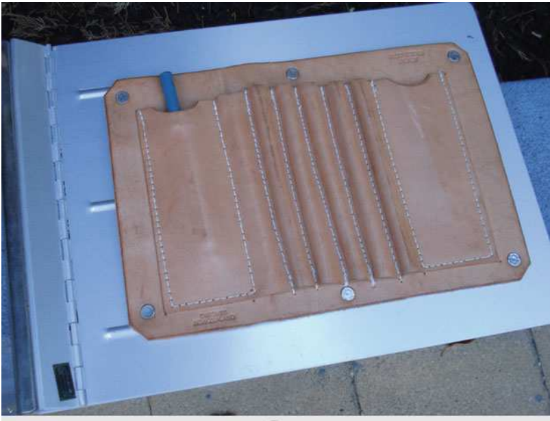
Fig. 3.10 Mapping sheets holder with attached pencils sheath for underground mapping
