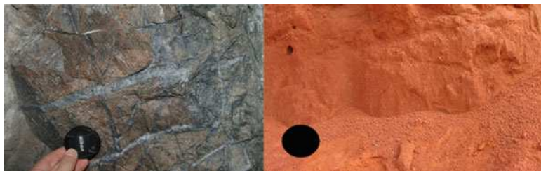
Fig. 9.1 Intuitive look on relationships between sample size, heterogeneity of the sampled materials and sampling error
