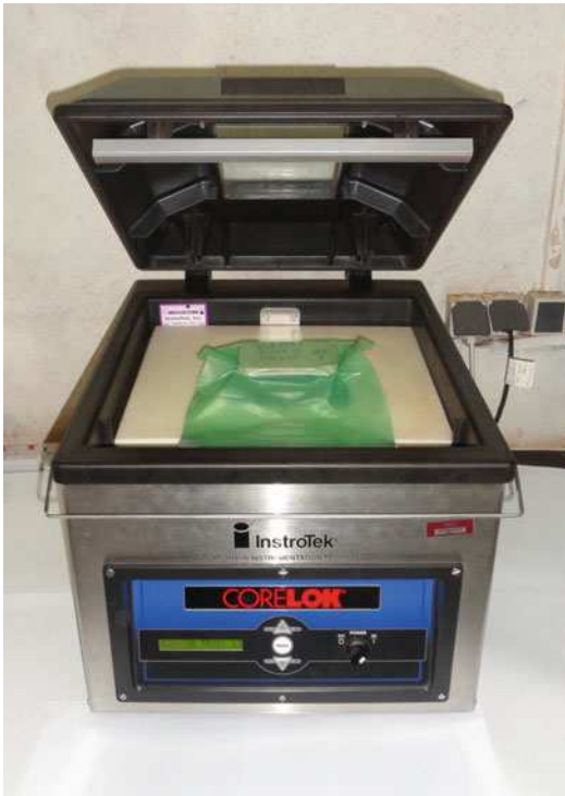
Fig. 7.2 CoreLok device for vacuum-sealing samples in the polymer bags
