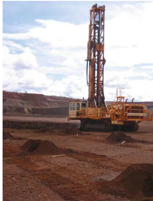
Fig. 4.21 Drilling blastholes using truck mounted open hole percussion drill rig, Yandi iron-ore mine, Western Australia
