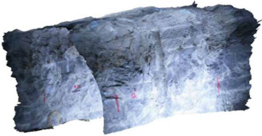
Fig. 3.18 Detailed 3D image of part of the underground drift (8 m long) recorded using ADAM photogrammetric technology, Diavik diamond mine, Canada
